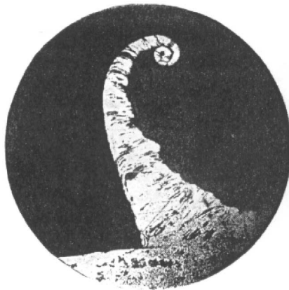
Fig. 2. Experimentally detected continuous chipping in ductile steels (Merchant, 1944).
